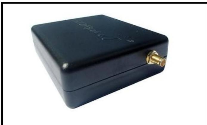
Want to play with a software defined radio? SDRplay is a receiver that features continuous coverage from 100 kHz to 2 GHz. It works with several popular SDR software programs on multiple platforms. Powered over a USB connection, and connected to an antenna it has performance that seems on par with conventional receivers. It is a step above the popular “stick” dongles in its wideband coverage and also has a series of band pass filters. And yes, those little, tiny parts do work.
